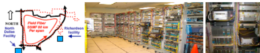
Figure 1: Left to right: Verizon 80km loop; Xtera 3040km all-Raman ULH system; Mintera 40 Gbps transponders
