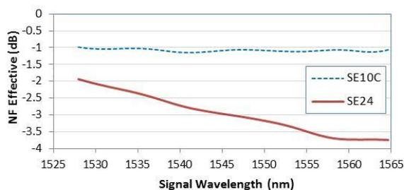
**Fig. 1.** Effective NF ( $NF_{BR}$ ) of Xtera's SE10C and SE24 across the C-band. The NF of an EDFA is about 4.5 to 5 dB (not shown).
