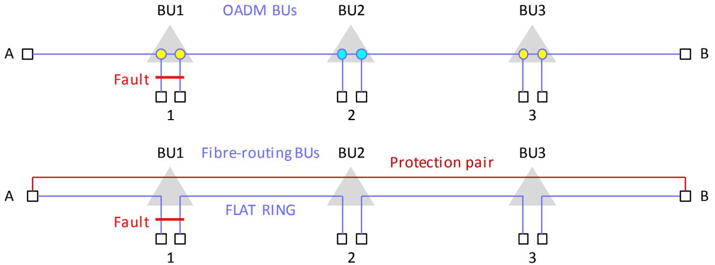
100 x 100G with 10-30 percent drop. This could be achieved with 100 x 100G and a ROADM BU, or with 120 x 100G and a fixed 30 channel drop, of which only a part might be used. The reduced losses of the fixed OADM BU will generally make the higher capacity possible without increasing the number of repeaters, thus producing a more cost-effective and simpler system. This solution, of course, becomes more difficult with larger drop ratios.
