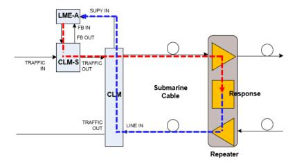
This allows the transmitted signal to be imposed upon the outgoing line data using Raman amplification. Such a scheme ensures little or no impact on the line signal, beyond the supervisory signaling itself, and ensures that the reliability of the LME-A does not impact upon the line data, i.e. the LME-A can be removed, for maintenance, from the SLTE without affecting traffic data.
