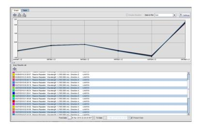
Measurements over any wavelength within the C-band can be made by the LME-P with dynamic switching to up to 10 different wavelengths being possible.
