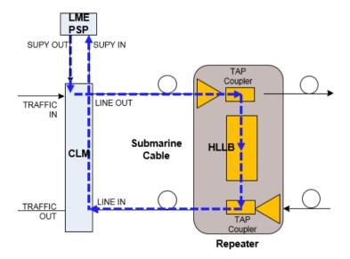
The transmitted signal traverses the cable section with portions being returned to the transmitting LME-P. The LME-P demodulates the returns from each HLLB and constructs a map of the fiber-pair which allows long-term monitoring of both the submerged plant and the interconnecting fiber.
