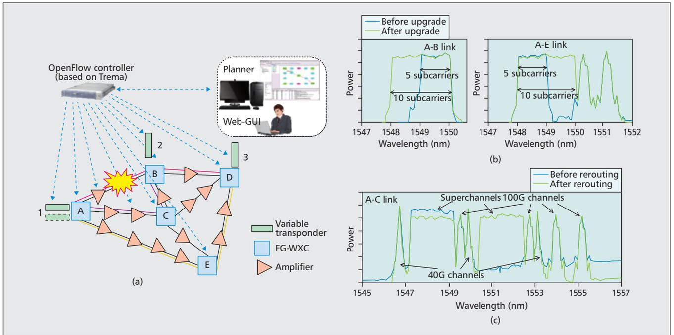
**Figure 7.** Demonstration of OpenFlow-enabled adaptive transport SDN.
