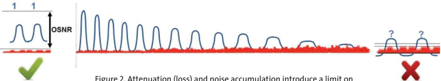
Figure 2. Attenuation (loss) and noise accumulation introduce a limit on transmission distance once the signal can no longer be reliably detected.
