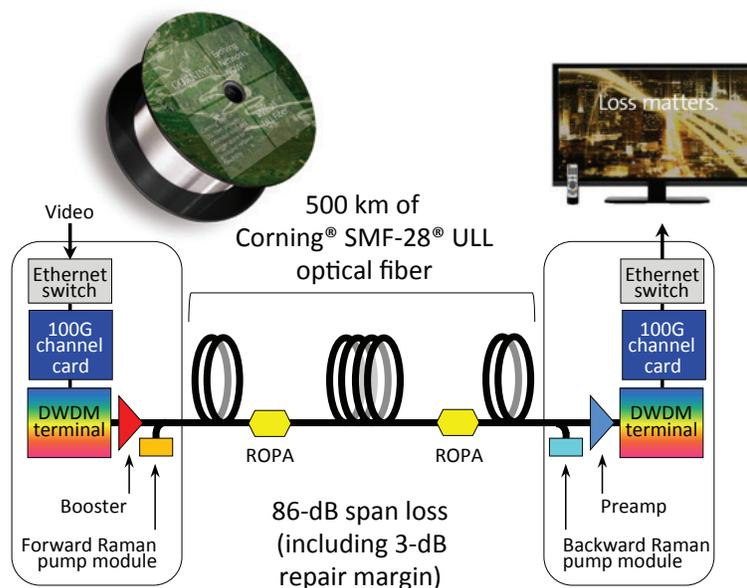
Figure 6. 100 Gb/s transmission over 500 km achieved by combining ultra-low loss fiber and advanced amplification technologies.
