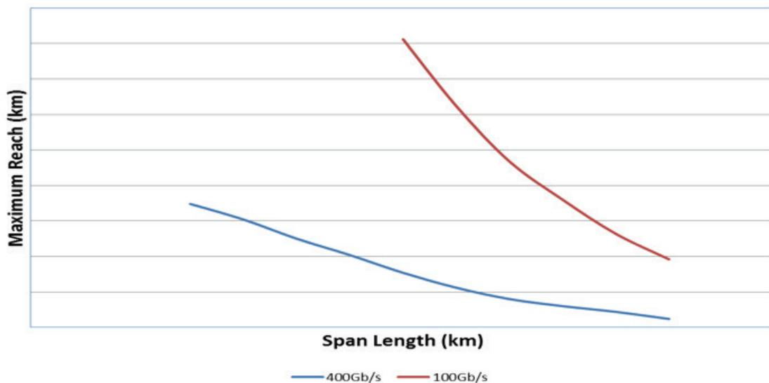
Figure 3. Achieving long reach without intermediate regeneration requires more frequent amplifier sites. This can force amplification sites in remote regions. Planning for 400 Gb/s requires even more frequent amplification.
