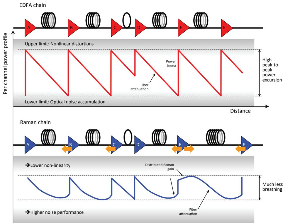
Figure 4. Typical per channel optical power profile as a function of the transmission distance in chains of EDFA and Raman amplifiers.
