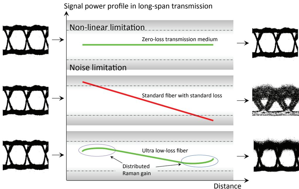
Figure 5. Advanced fiber and amplification technologies to minimize optical signal attenuation along the optical path.
