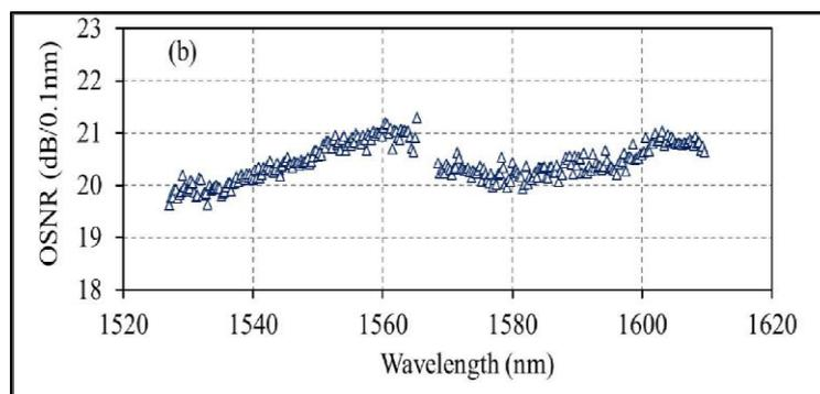
Figure 1 OSNR versus Wavelength for C+L lumped amplifiers (Cai et al<sup>2</sup>)
