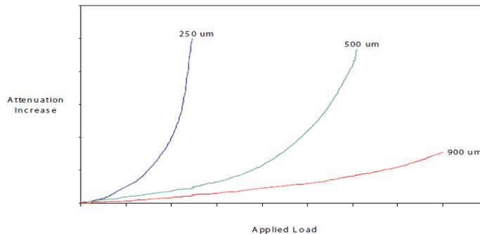
Figure 2 Effect of Coating thickness on micro-bending (Note that the cladding size is 125micron)
