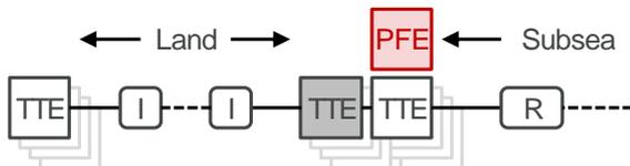
Figure 2: Equipment for re-transmission [ I = In-Line Amplifier (ILA) ]
