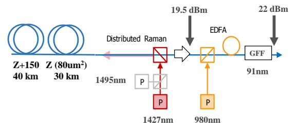
pumps (one 980 nm, two 1427 nm and two 1495 nm) to obtain a continuous amplification gain in the C+L bands, between 1525 nm and 1616 nm, as Figure 1 shows. The pump powers were varied up to 650 mW for the 980 nm pumps and up to 310 mW for the Raman pumps.
