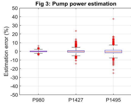
The two extreme errors at around 24 % and 38% for the 1427 nm and 1495 nm Raman pumps are owing to the NN not perfectly matching on two data sets. These errors might well be improved with additional training data.
