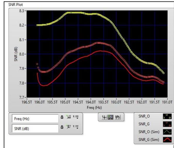
**Fig. 3.** Case A recalculated SNR values. Lines are from simulation and symbols are from  $SNR_G$  equation.
