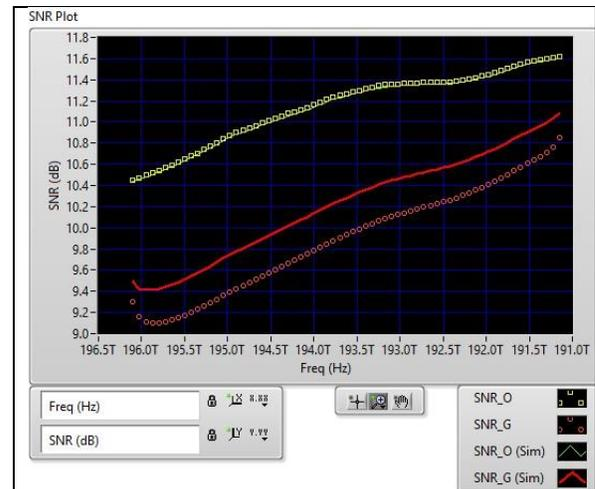
**Fig. 4.** Case B recalculated SNR values. Lines are from simulation and symbols are from  $SNR_G$  equation.
