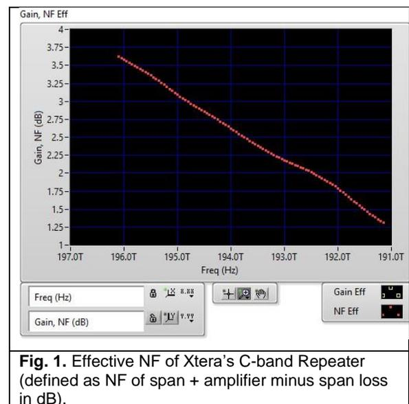
**Fig. 1.** Effective NF of Xtera's C-band Repeater (defined as NF of span + amplifier minus span loss in dB).
