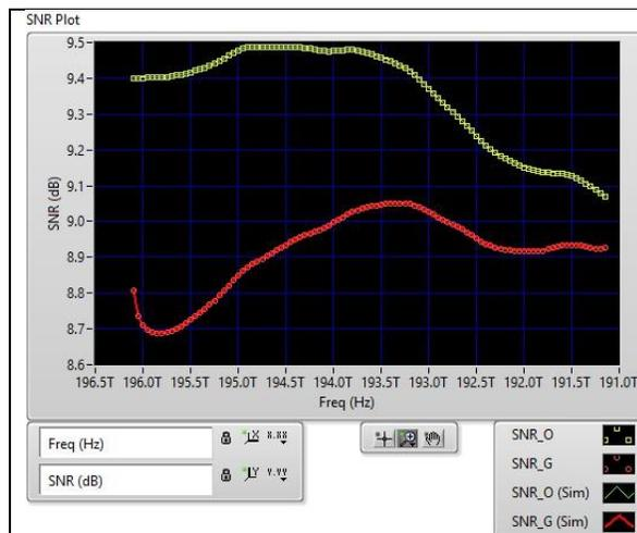
**Fig. 2.** Baseline link simulation. Lines are from simulation and symbols are from  $SNR_G$  equation.
